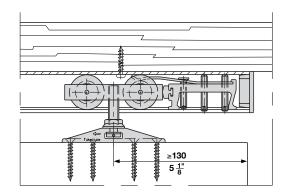
The two-way suspension bracket allows the door leaf to be hung and to be taken off in two different ways:
